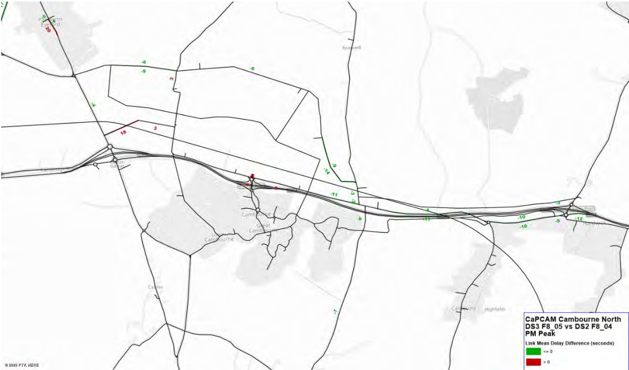
Figure 33 - DS3-DS2 Link Delay Difference - PM Peak Hour
