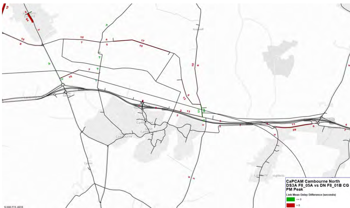
Figure 35 - DS3A-DN Link Delay Difference - PM Peak Hour
