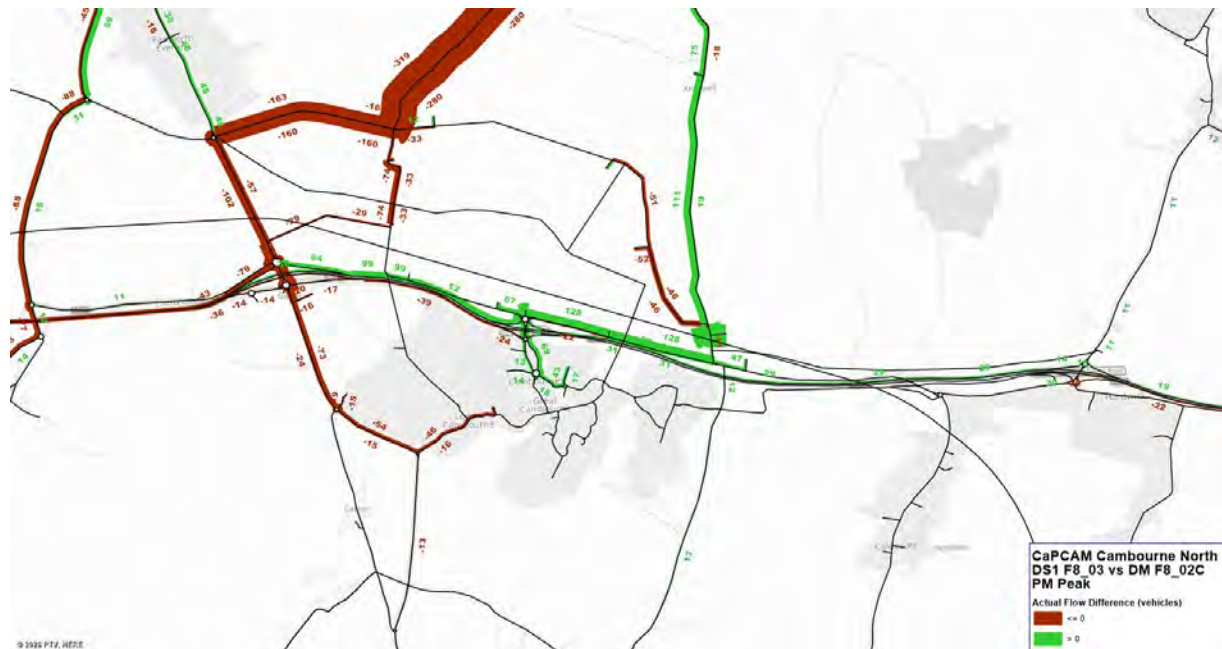
Figure 19 - DS1-DM Link Actual Flow Differences - PM Peak Hour
