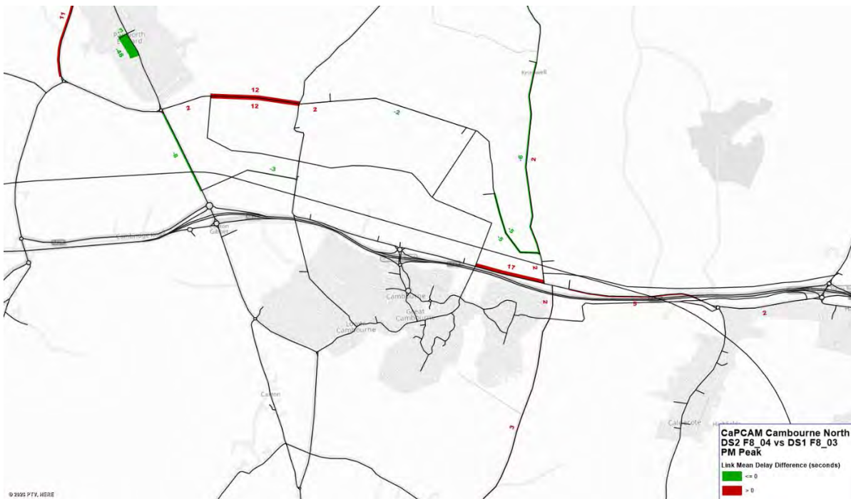
Figure 31 - DS2-DS1 Link Delay Difference - PM Peak Hour
