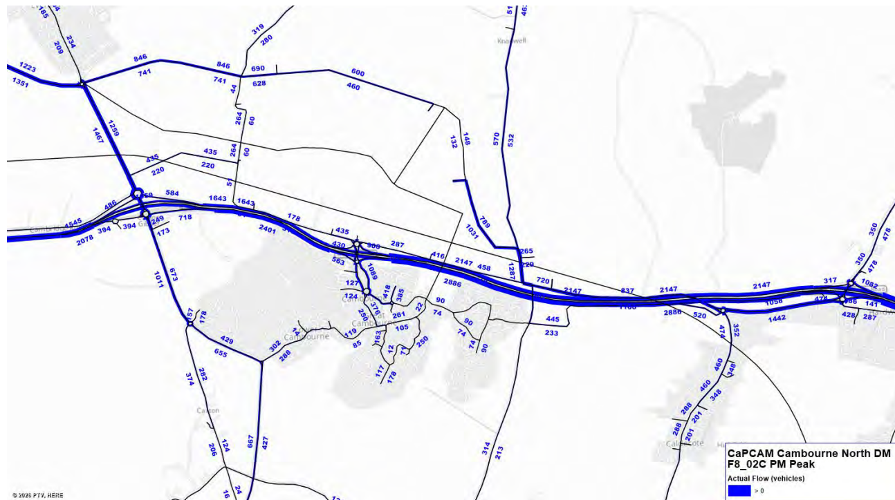
Figure 9 - Cambourne North DM - Link Actual Flow PM Peak Hour
