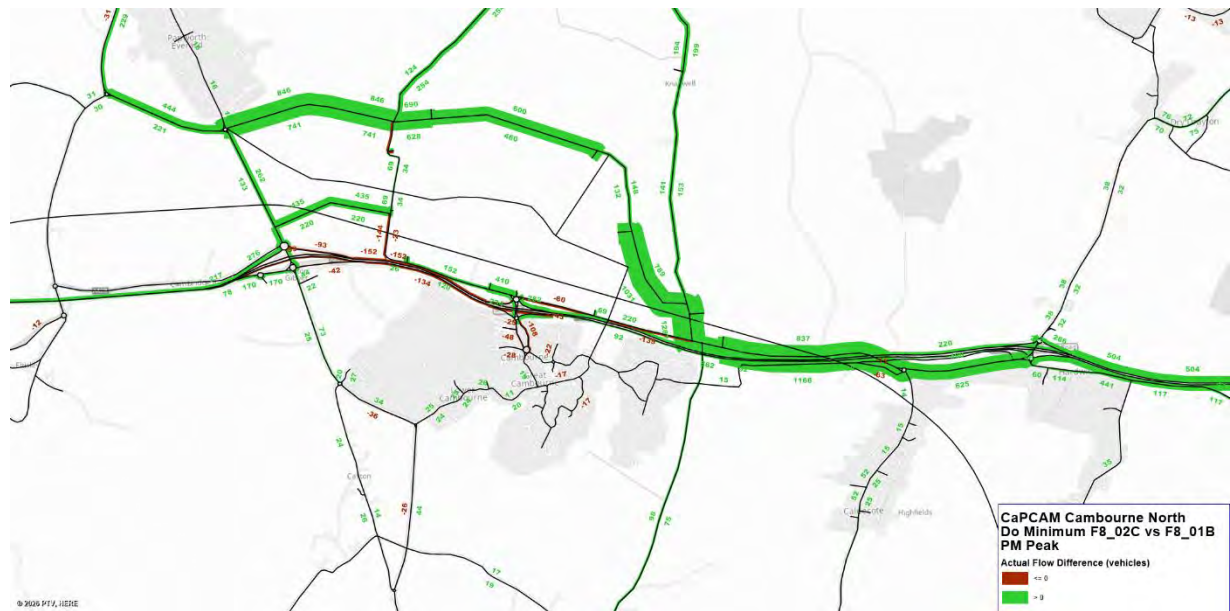
Figure 17 - DM-DN – Link Actual Flow Differences - PM Peak Hour
