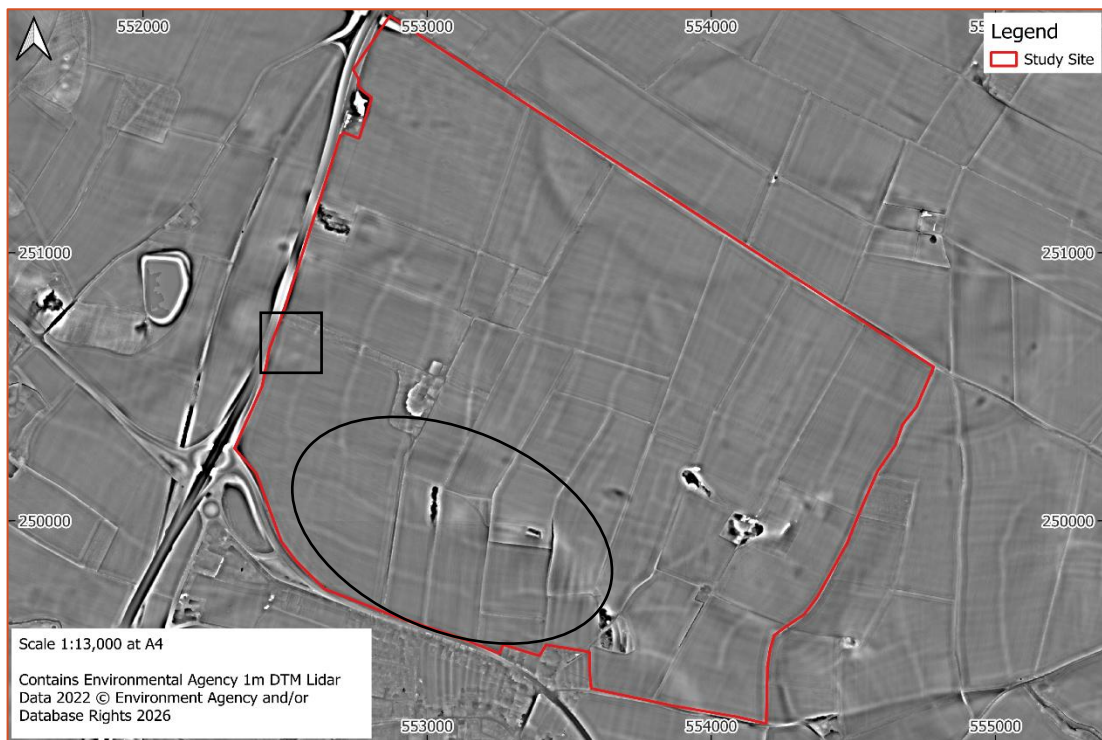
Plate 15 1m DTM Lidar data rendered using RVT Simplified Local Relief Model
