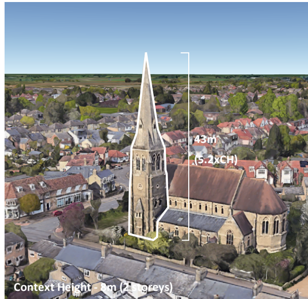
Image 41: Super Tall Building - Context Height Ratio 5.2, St. Luke's Church, Cambridge © Google Earth
