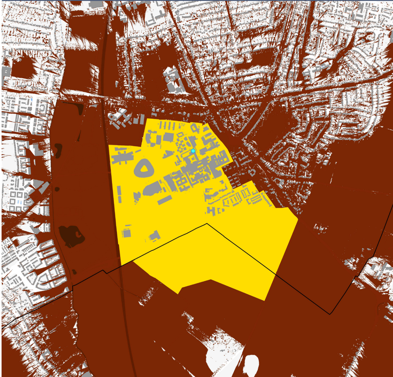
Viewshed Analysis for Area of Search with development heights of 30.5m and 25.5m (Tall building threshold + 6.5m (2 Storeys))
