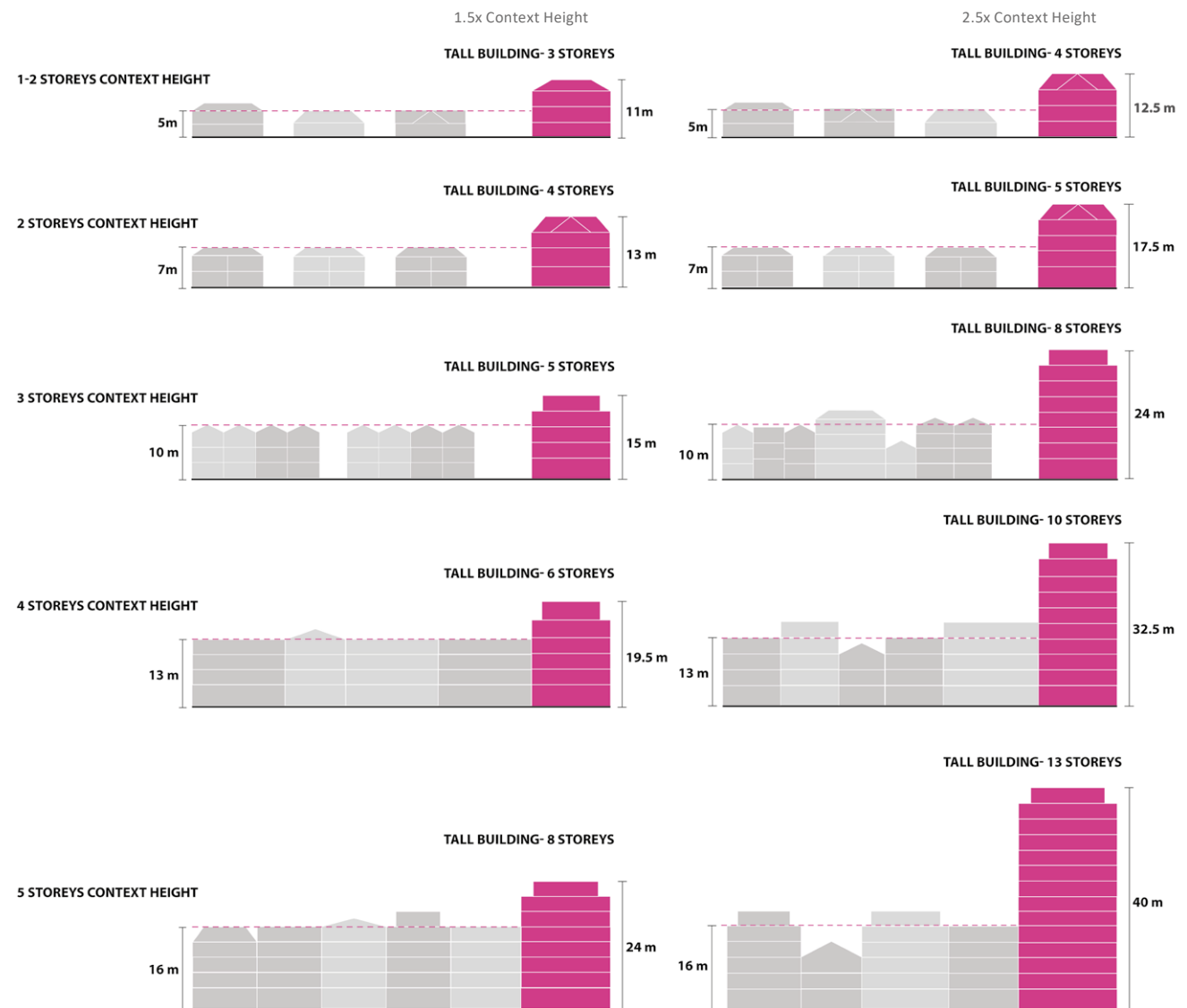
Figure 4: Diagram illustrating local landmarks relative to their context height (1.5x and 2.5x context height)
