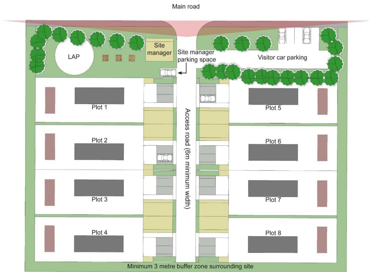
Figure C2: Illustrative layout for a site of 8 pitches (with key)
