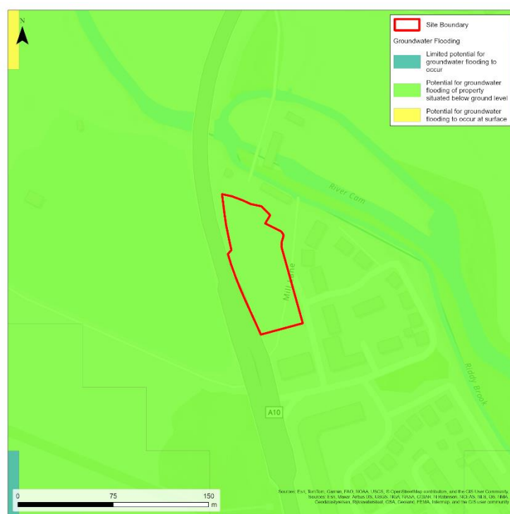
Figure 121: Susceptibility to Groundwater Flooding Map
