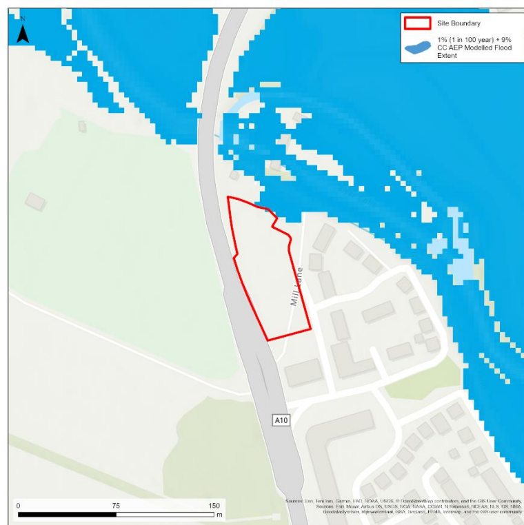
Figure 118: Modelled Fluvial Flood Extent (1% AEP with Climate Change)
