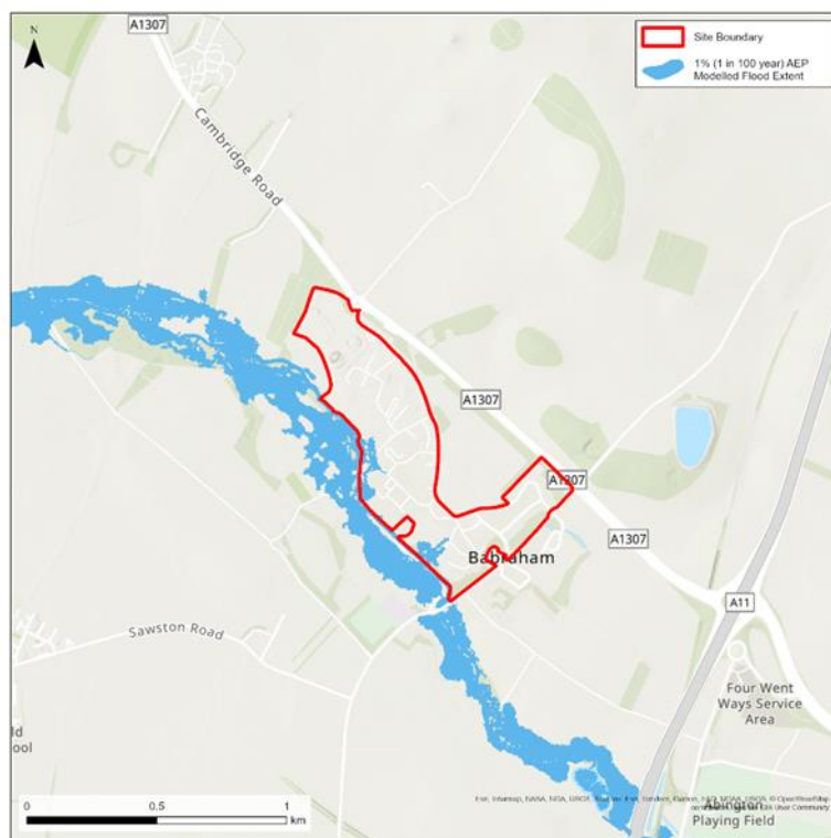
Figure 63: Modelled Fluvial Flood Extent (1% AEP)
