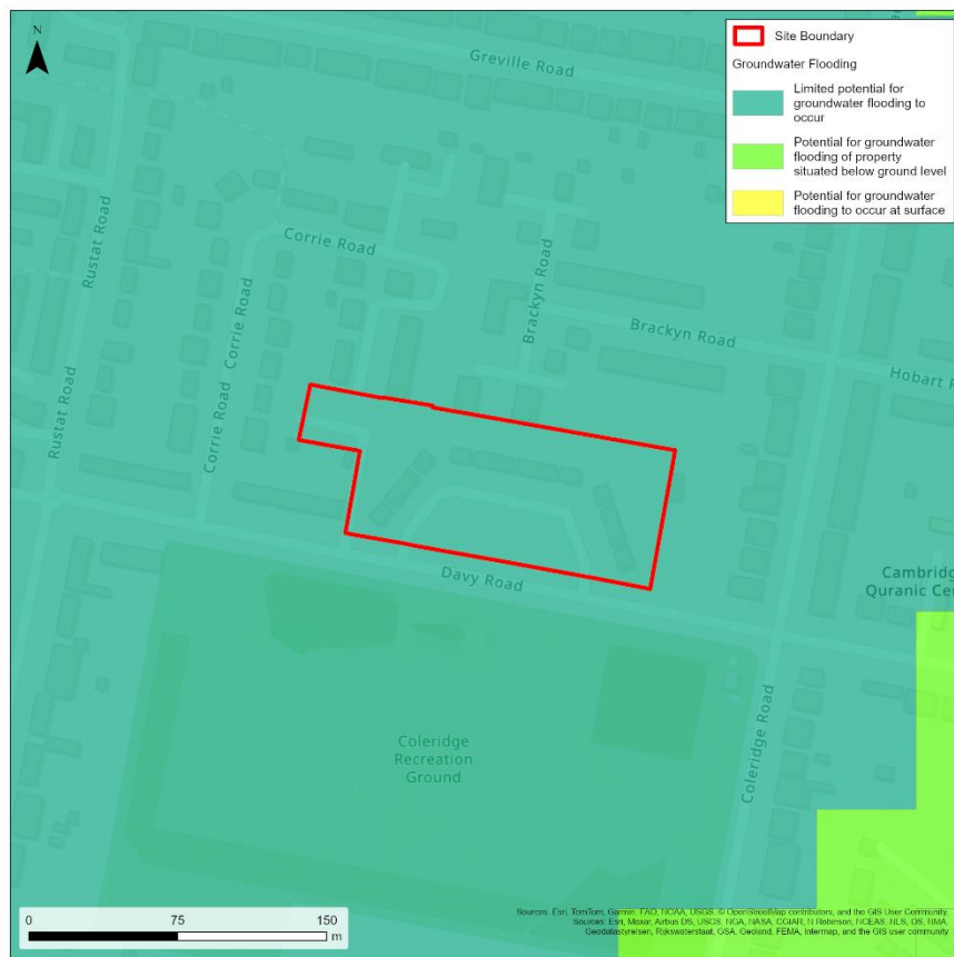
Figure 53: Susceptibility to Groundwater Flooding Map
