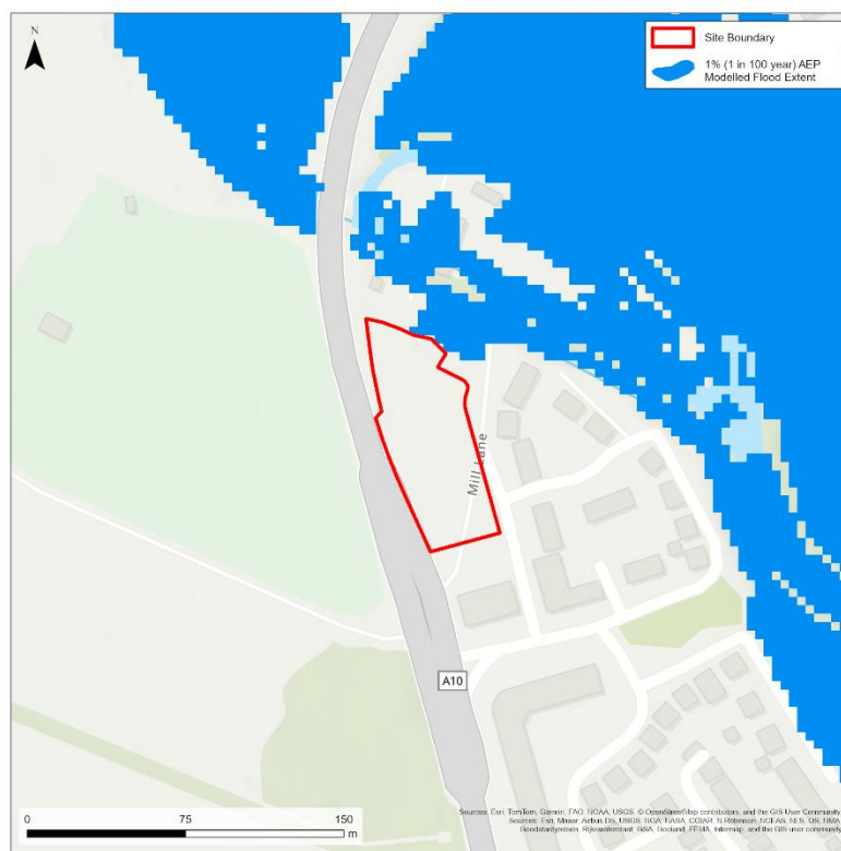
Figure 116: Modelled Fluvial Flood Extent (1% AEP)
