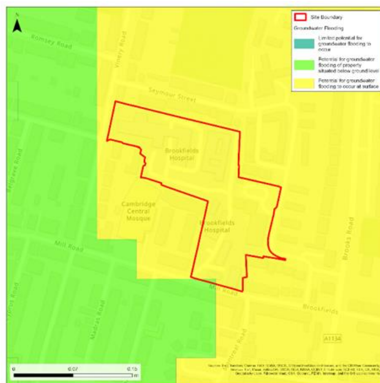
Figure 58: Susceptibility to Groundwater Flooding Map
