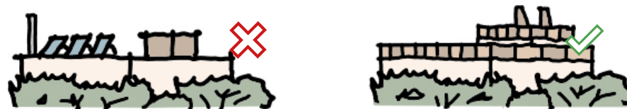
Figure 62: Development should discretely integrate solar panels, lift overruns, plant rooms, exhaust stacks, cranes, telecommunication and other equipment within the overall envelop of the building. They should be a constituent part of the architectural expression. This can be achieved for example by screening equipment behind parapets, or articulating exhausts stacks as deliberate vertical architectural features.
