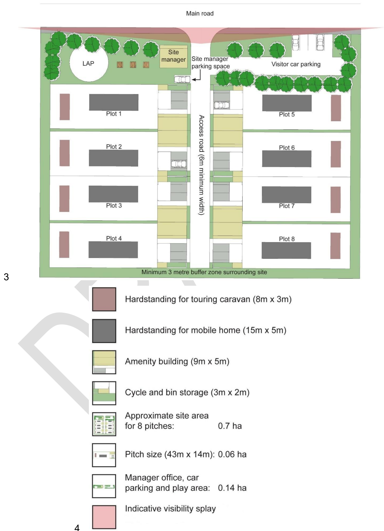
Figure 2: Illustrative layout for a site of 8 pitches (with key)
